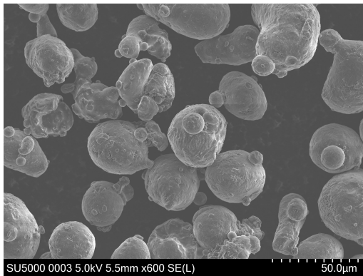
Figure 1: AlSi10Mg powder by ECKA. PSD: 20-56 μm. SEM magnification: 600x.
